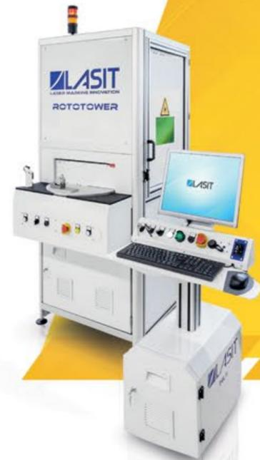
The **RotoTower** laser marker has two-position index table with a **20 mm-thick Fibral aluminium disc**. The disc has 2 centring holes for the templates and 2 threads in correspondence with the two stations. The holes are  $\varnothing 8H7$  with hardened bushes and the threads are M6 with Helicoil.
