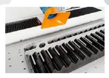
With a maximum marking area of 750x450 mm using the focal FFL254, laser marker CompactMark G7 can mark small pieces but also a pallet with hundreds of pieces.
