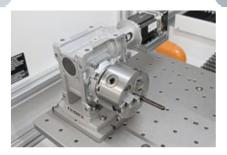
In the standard configuration, Compact G7 has 3 axes, but it's possible to add W axes and rotary head, in order to make the machine suitable for more applications.
