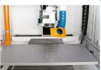
The heart of the machine is the XYZ axes, which is a single unit sustained by the external Bosch profile structure. G7 is not the simple combination of 3 axes, It's a real laser working system designed with FEM technics.
